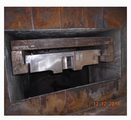
Finally in Nov'14 opportunity shutdown, DDSV-1 was inspected & found derailed from its position, which was replaced with help of M/M.
